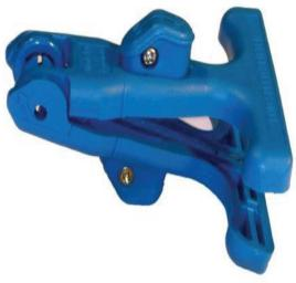
Developed specifically for technicians working with flat drop cable, the SPEEDSLITTER™ opens cable jacket easily and safely with one pull. A simple twist of the cable allows the jacket and strength members to separate from the buffer tube leaving the fiber undamaged. Snip off the separated jacket and splice. Works on most flat fiber drop cable.
